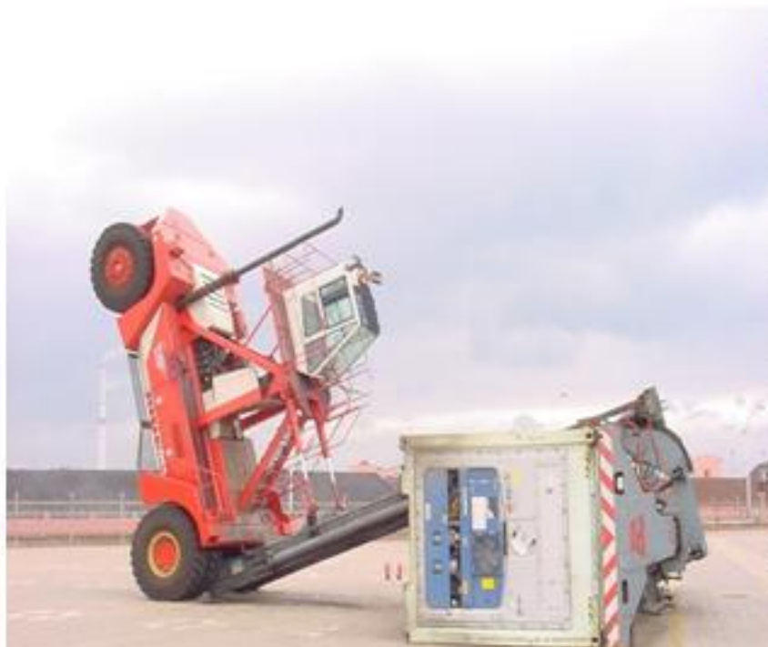
Lift truck tipping forward
